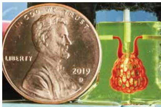
A U.S. penny is shown next to a scale model of a lung-mimicking air sac with airways and blood vessels.
